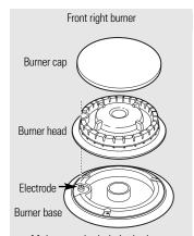
Make sure the hole in the burner head is positioned over the electrode and that the burner head is fully inserted inside the burner base.
